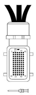
The above is the schematic diagram of overload connector and metal contact pin
