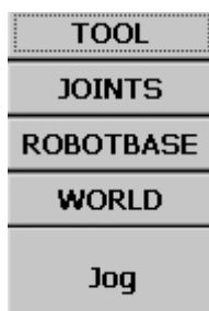
Figure 12 Jog Reference Coordinate System Setting
